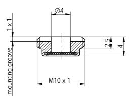
Plug type VSCH- M10 x 1/WD (with sealing)
